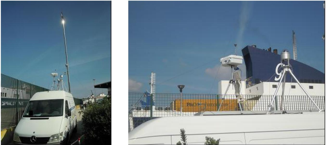
*Figure 3. Left: Photo showing the Mobile Laboratory ISAC – CNR located at the passenger terminal., Right: Photo of the sensors installed on the roof of the Mobile Laboratory*
